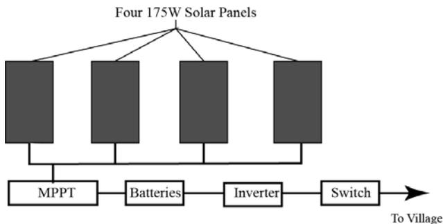
Figure 1: Wiring diagram of solar array.
