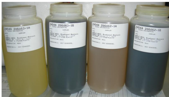
Figure 4. Output samples from the portable biodiesel system
