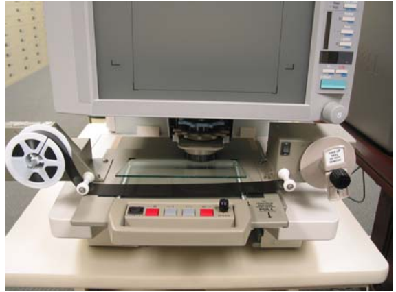
This is the powered advance microfilm reader. Notice the buttons and knobs.
