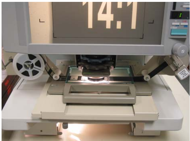
3. Tray retracted and ready for use. Notice the lens is over the microfilm.
