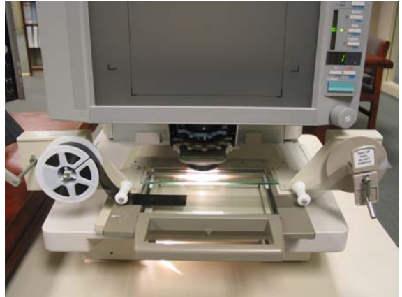
This is the manual advance microfilm reader.
