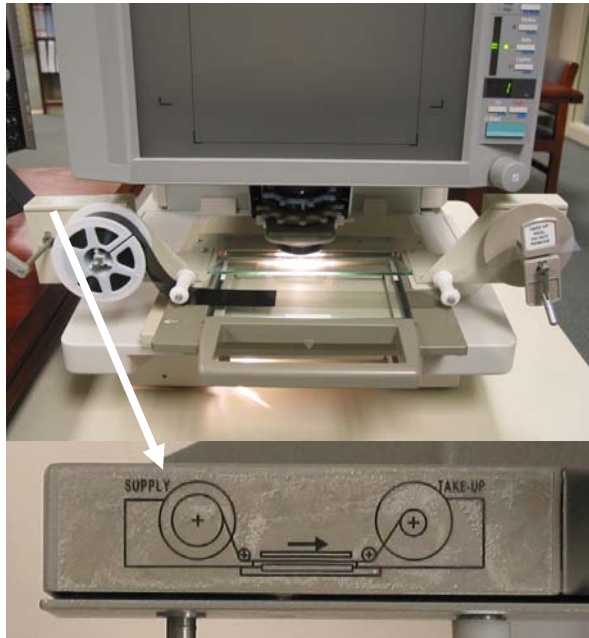
2b. This is a top down view of the loading instructions on the Supply (left) reel holder.
