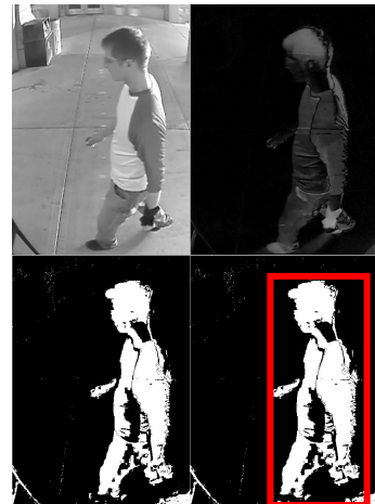
Image processing example: grayscale, subtraction, threshold, and tracking
